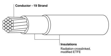
SPEC 55 Insulation System—Single Wall
